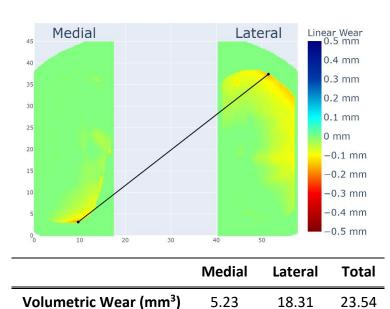
The angle between the centre of the medial and lateral wear scars was 39° (39° internal rotation).
